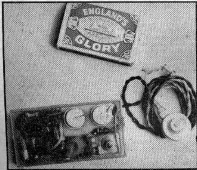
This photograph shows the compactness and extremely small size of the 3-transistor receiver built by the author and described here-with.
