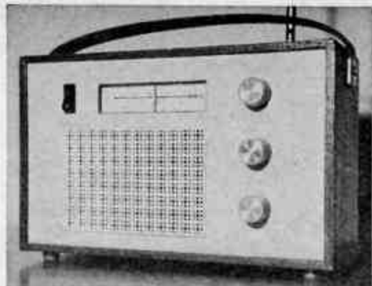
The exceptionally neat and symmetrical layout of the author's receiver is well demonstrated by this photograph. To the left of the tuning scale is on-off switch S1. The three controls to the right are (from top to bottom) tuning, regeneration and a.f. gain
