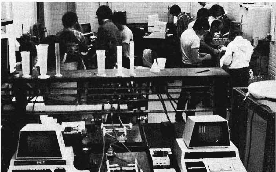
University of Rochester Chemical Engineering students during a laboratory session. The three computers in the foreground are each being used with a separate experiment to make temperature measurements. Each of the four computers in the background are interfaced to gas chromatographs and are being used for data acquisition and analysis. Both applications involve the QM-100-amplifier combination discussed in the text for A/D conversion.
