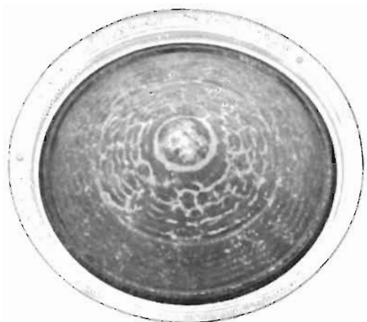
Fig. 9. Photograph of a vibrating speaker. The outer portion of the cone is "at rest"; the frequency fed to the speaker is about 3500 c/s. (See p. 5).
