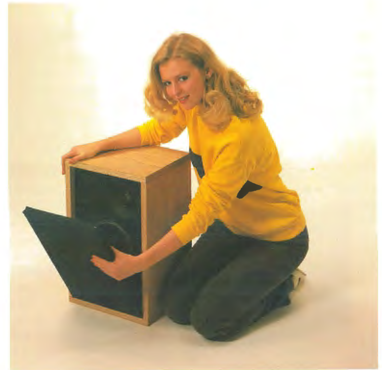
Fitting the grille cloth frame inside the front recess.
